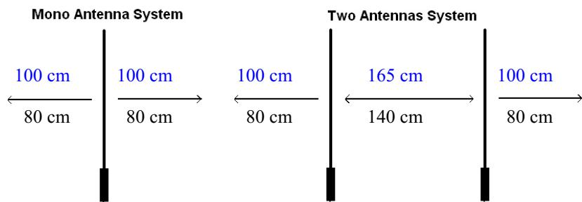
**When tag is in the position of the best detection the maximum detection range**
